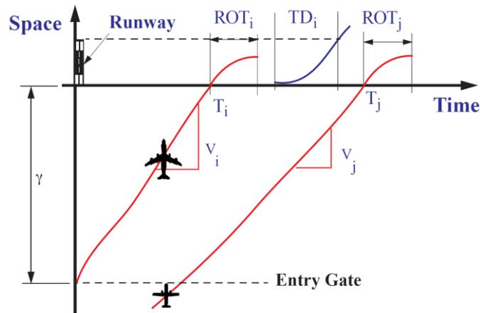
Fig. 2: Occupancy of time-space in runway occupancy time for landings and in take-off distance for departures on a mixed mode single runway (Trani, 2005; [http://128.173.204.63/courses/cee3604/cee3604\\_pub/Time\\_space\\_diagrams\\_cee3604.pdf](http://128.173.204.63/courses/cee3604/cee3604_pub/Time_space_diagrams_cee3604.pdf)).
