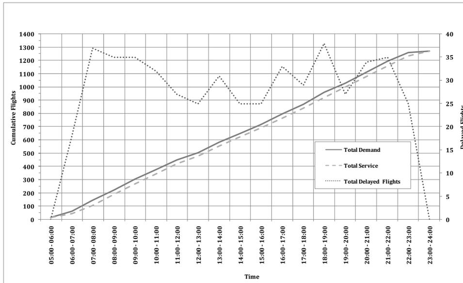
Fig. 6b: Cumulative diagrams of Berlin-Brandenburg International (BBI) airport 100% growth scenario simulation output
