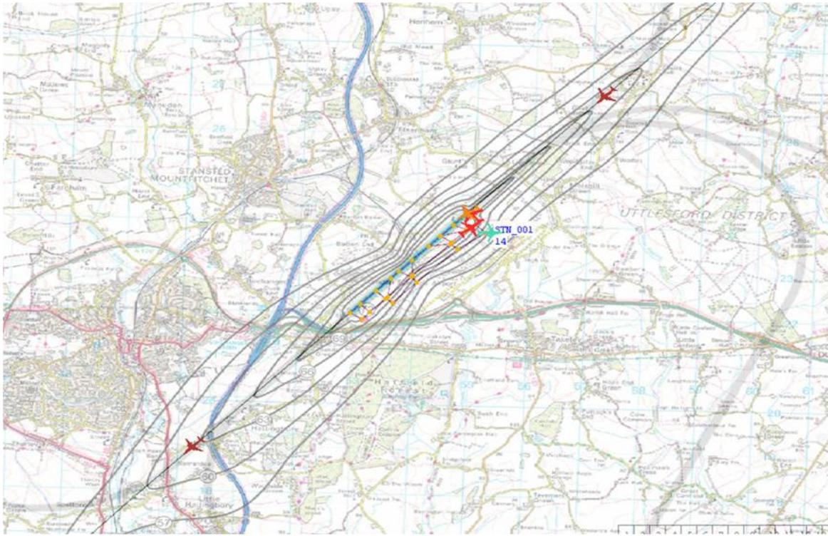
Fig. 7: Overlay of Noise and Population maps on airside traffic animation (and associated departure queue) at Stansted airport
