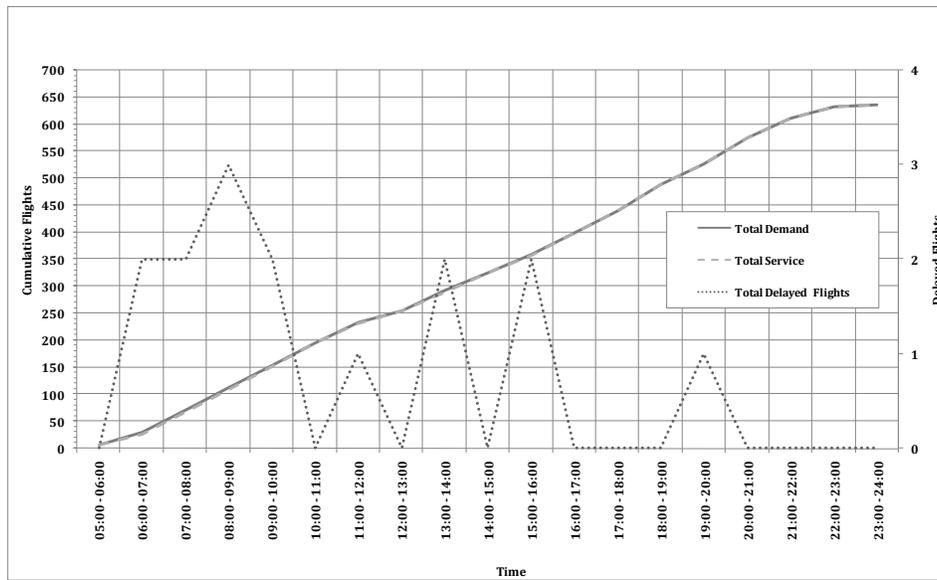
Fig. 6a: Cumulative diagrams of Berlin-Brandenburg International (BBI) airport baseline simulation output
