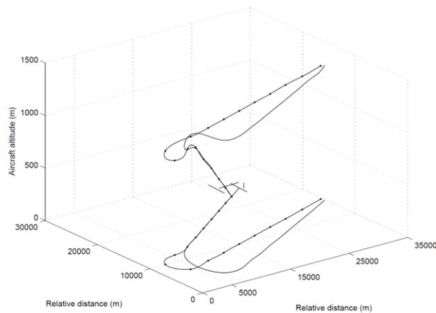
Fig. 1: Paths of two subsequent flights at Amsterdam Schiphol in 3-D space and as 2-D ground projection (Swart, 2003; <http://www.math.leidenuniv.nl/scripties/Swart.pdf>).
