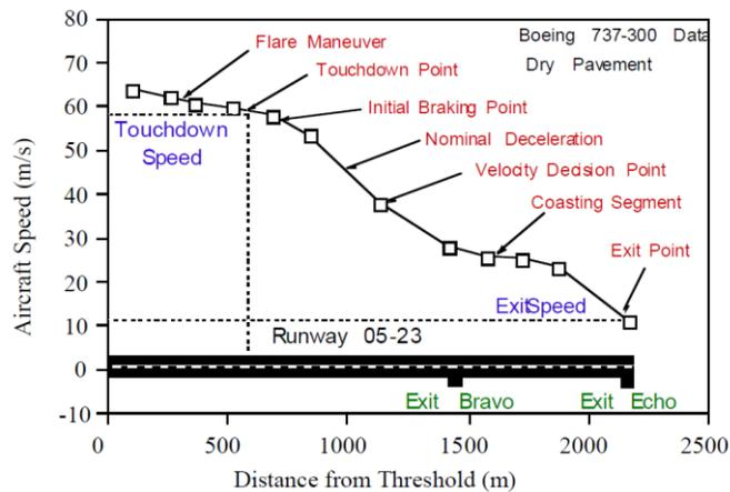
Fig. 3: Deceleration speeds during phases of a landing on a runway (Trani, 2000; <http://www.nasug.com/200009/rot.pdf>)
