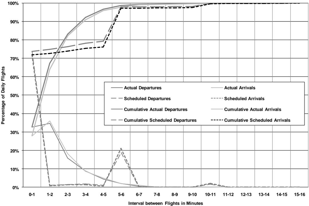
Fig. 5a: Scheduled and actual interval times of flight at London-Heathrow airport
